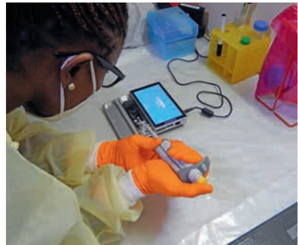
Loading samples on a nanopore-based sequencing device
